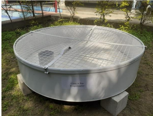
Class A Pan Evaporimeter
