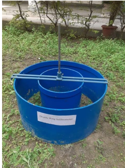
Double Ring Infiltrrometer
