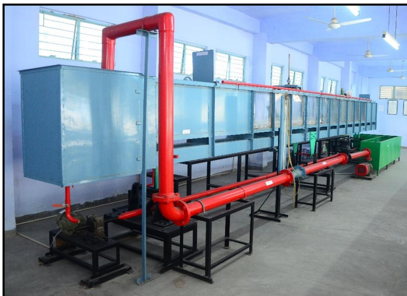
Open Channel Flume
