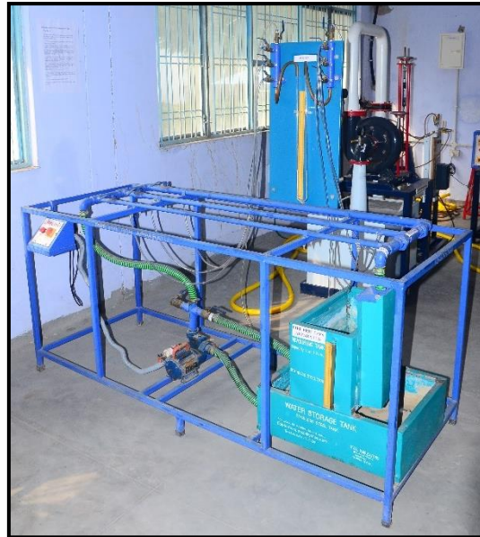
Pipe Friction Apparatus
