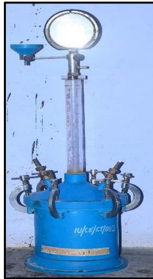
Concrete Air Entrainment Meter Apparatus
