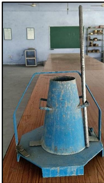
Slump Test Apparatus
