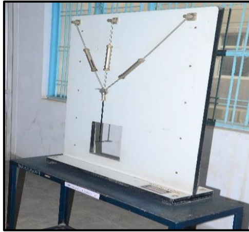
Redundant Joint Apparatus
