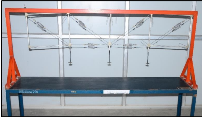
Deflection of Truss Apparatus.
