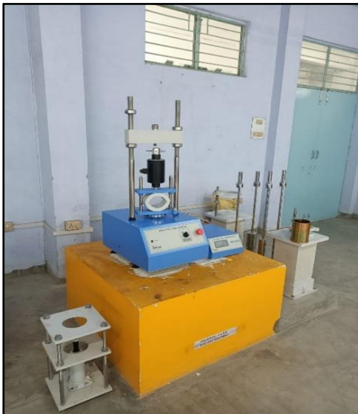
Marshall Stability Testing Machine and Marshall Compactor
